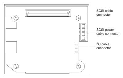
**Note:** To install an additional hot-swap drive backplane on the back of the server, see "Installing a 3-Pack Ultra160 Hot-Swap Expansion Kit" on page 71
